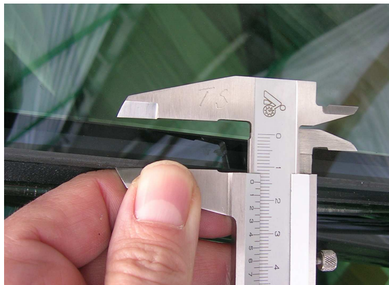
White Lines at the Edge Bond of a Solar Protection Glass Pane
